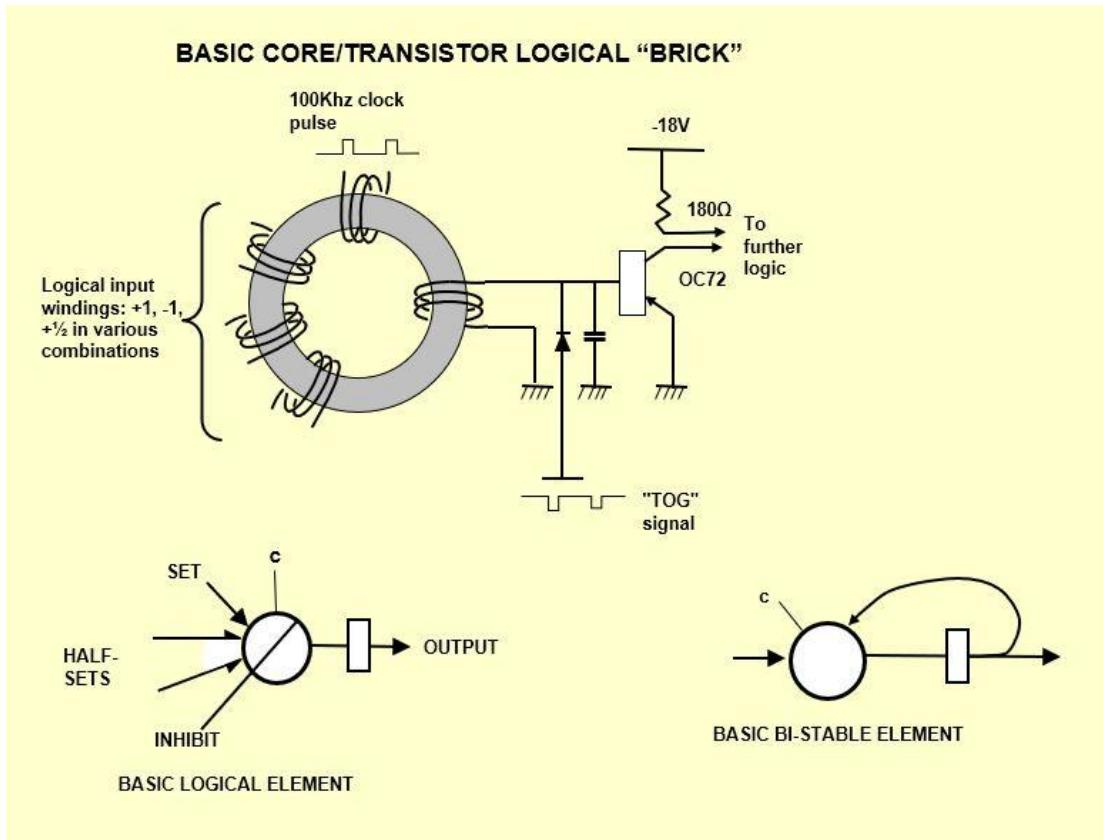
The ferrite ring, which I shall refer to as a "core" (because it's fewer syllables and time is short), is the same as was used for data storage in machines of this generation. It is about 2mm across (0.08") and can be magnetised in either direction, clockwise or anticlockwise as we look at the picture, and the state of magnetisation remains until it is changed by current through one of the windings. We can talk about the core being "set" or "unset", depending upon which way it is magnetised.
